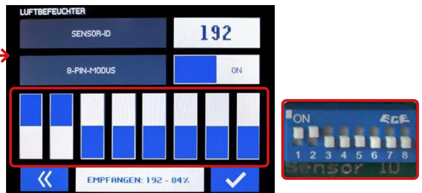
Fig. 5.6.7: Coding radio humidity transmitter
