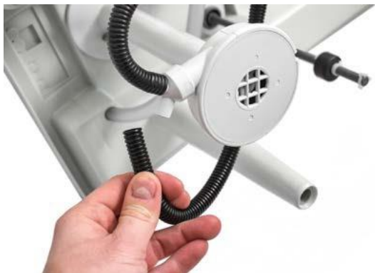
Fig. 7.4.1.5: Pulling off the pump hoses
