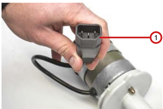
Fig. 7.4.1.7: Loosening the plug connection
