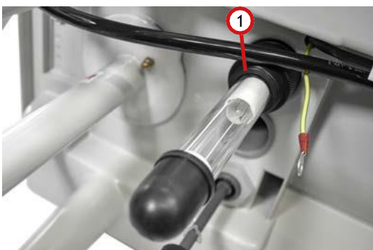
Fig. 8.1.2.6: UV lamp in quartz glass tube.
