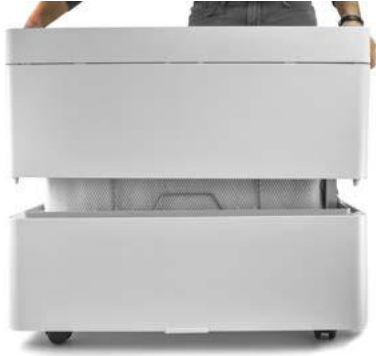
Fig. 6.3.2.1: Removing the upper part of the housing
