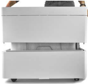
Fig. 6.3.4.1: Removing the upper part of the housing
